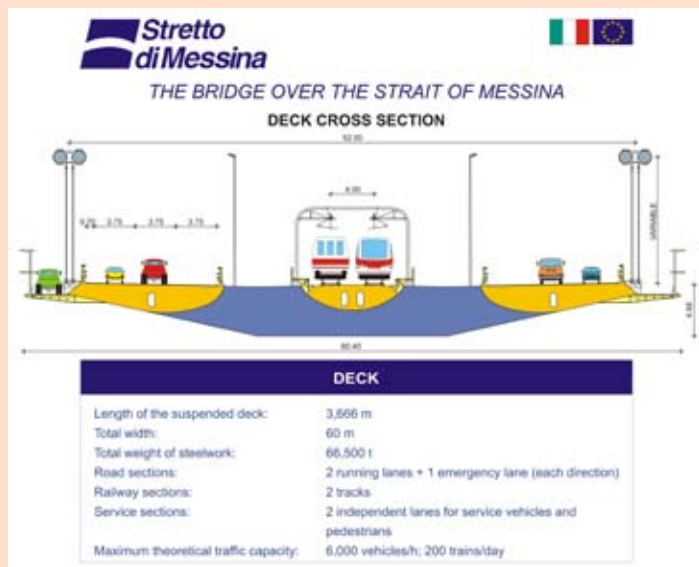
Fig.4: Cross-section of the deck.
